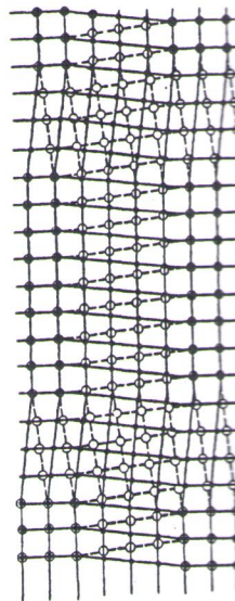
Figure 13.10. A pure (relaxed) twist grain boundary is in the plane of the figure. The boundary is normal to the boundary. The boundary in one grain and the solid surface have been relaxed to regions of poor matching (B), w
